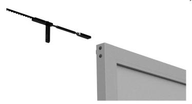
Manually pull the belt connection assembly towards the open position until the hardware is clear of the panel to be removed.
