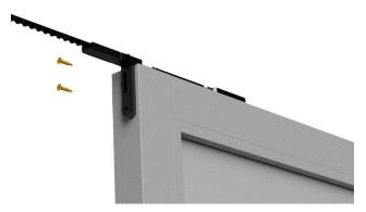
Place the 1/4" pin panel bracket into the turnbuckle on the top of the lead panel Pre drill 1/4" pin panel bracket using a 3/32" drill bit
